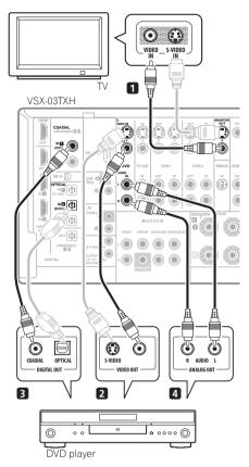
The diagram shows a basic setup of this receiver together with a TV and DVD player, with S-Video or composite video connections. Different TVs and DVD players may offer alternative connections. See also Using the component video jacks on page 19 if your TV and/or DVD player has component video inputs/outputs. If your DVD player offers multichannel analog audio outputs, see Using XM Radio on page 56.
